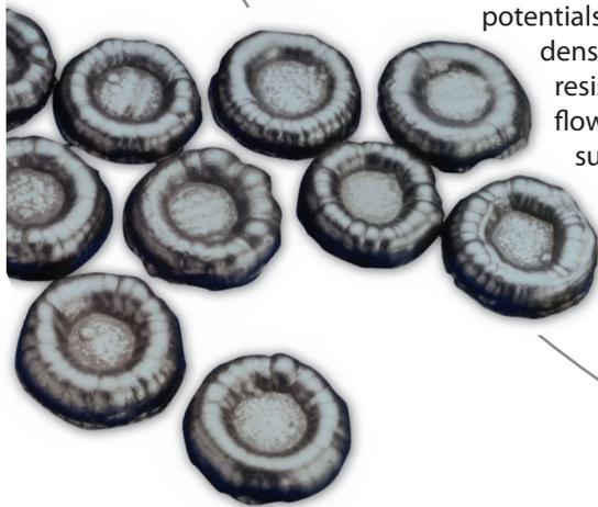
The lower resistance to current flow compared to sulfur-free nickel accounts for significant power and cost savings in the plating shop.
